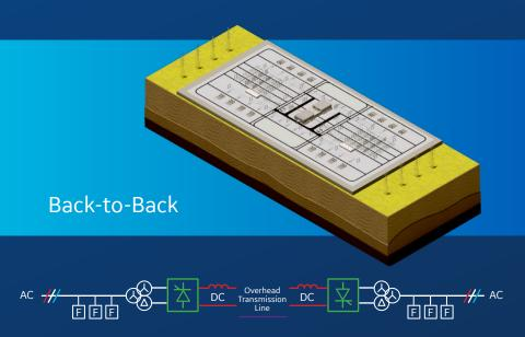
Suitable for frequency changing and asynchronous connections. This scheme provides fast accurate power flow, limiting the spread of cascading faults and provides increased system flexibility and prevents the need to build a new generation network. Once interconnected, the two systems' daily and seasonal cost differences can also be optimized.
