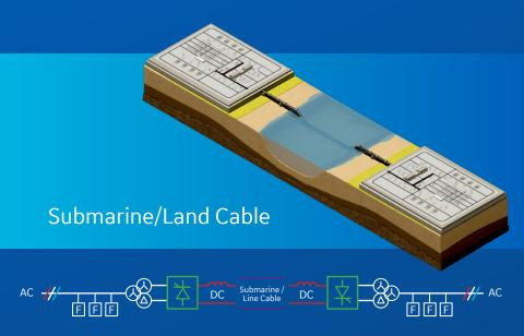
Where the power exchange or transmission crosses water, or an environmentally sensitive region, cables may be the favored method of interconnection between the HVDC Converter Stations. HVDC transmission is particularly attractive and may be the only technically feasible method of transmitting power using cables.
