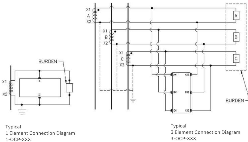
A Current Transformer secondary should never be open circuited while the Current Transformer primary circuit is energized. If this situation should occur there is a possibility of developing extremely high voltages which could be dangerous to personnel or cause an insulation breakdown.
