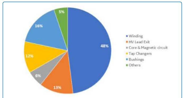
**Figure 2:** Major failures location for HV generator transformer > 100 kV, acc. CIGRE WG 2.37 - Transformer Reliability survey 2015
