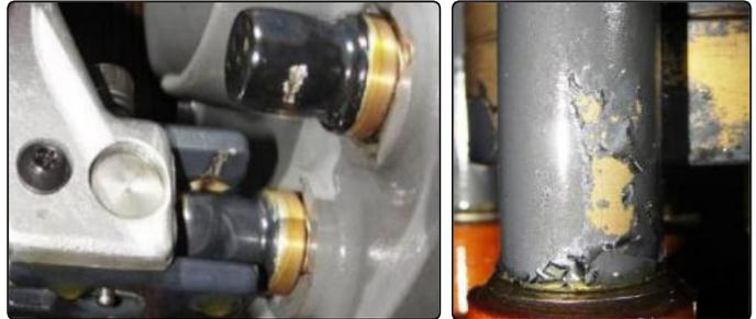
**Findings:** Silver sulphide on de-energized tap changer of a large 35 year old 330 kV/138 kV/11 kV auto-transformer.
