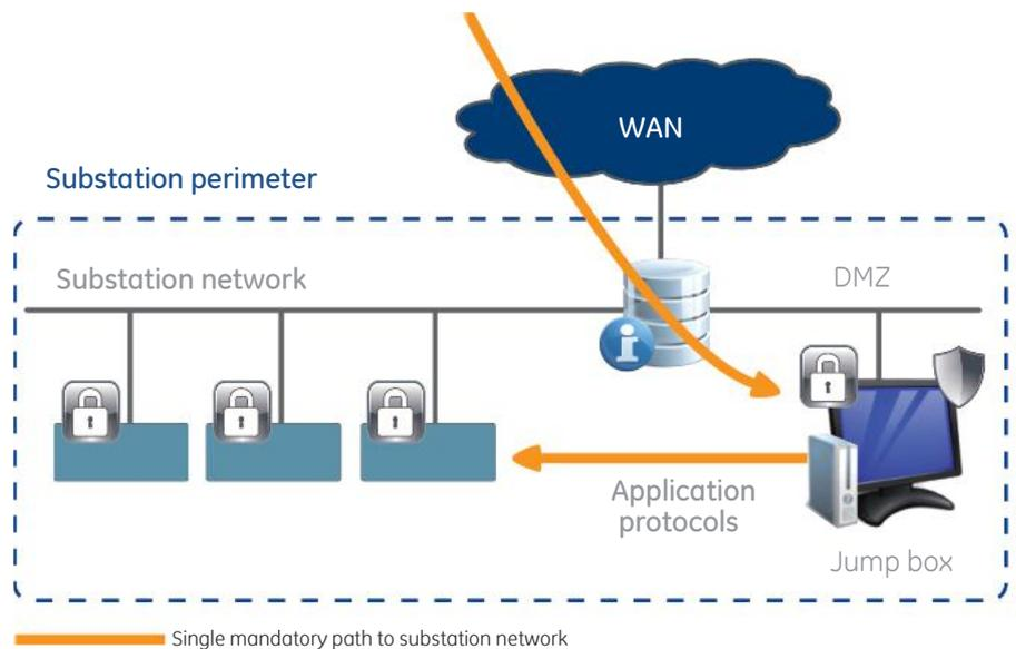
To protect the automation system configuration and setting files, integrity control software is added. The remote access to the substation has to be done first through a jump box installed in the substation DMZ which has access to the substation network. It is used to access the critical elements of the operational network. These elements are protected against attacks with hardening, whitelisting, memory protection and file integrity.
