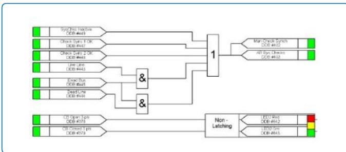
Figure 7 Programmable scheme logic
