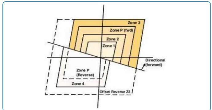
Figure 5 Quadrilateral characteristics
