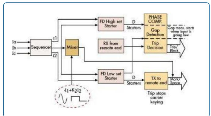
Figure 2 Phase comparison protection functional diagram
