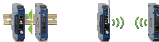
Expansion modules connected via backplane
