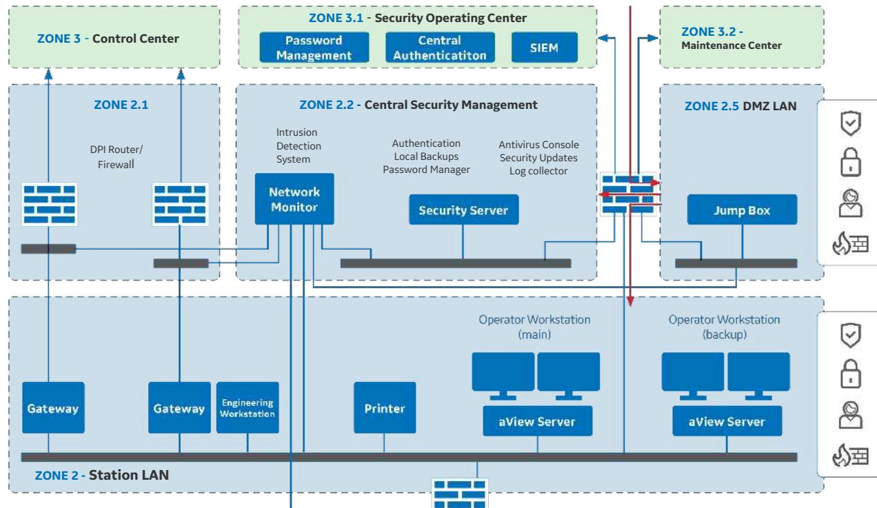
Figure 2: Router forwarding external communications to DMZ
