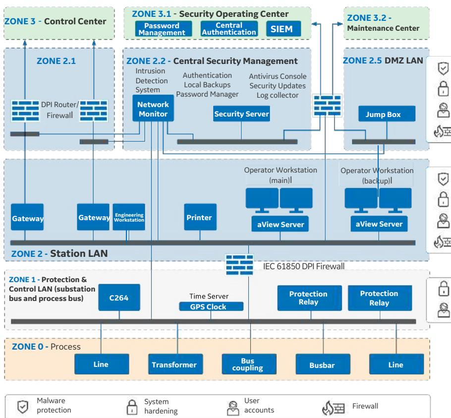
Figure 1: Secure Architecture
