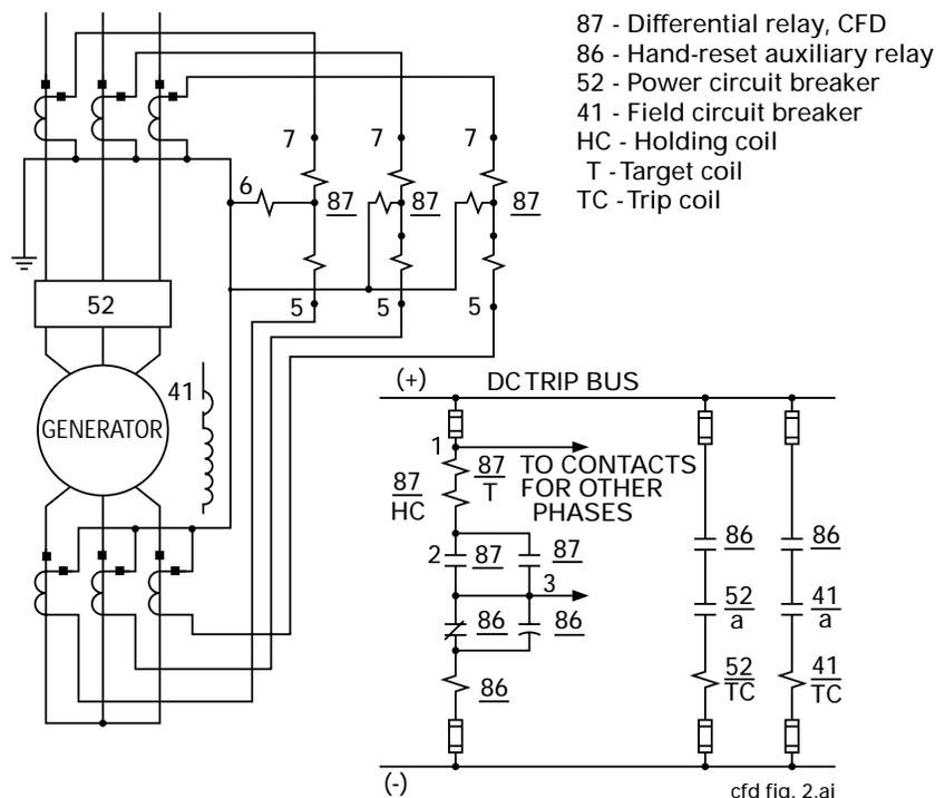
coils produce an operating torque that is proportional to the product of these two currents and the cosine of the angle between them. These are the conditions that will exist during an internal fault when part of the fault current comes from the bus.
