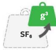
Replacing 1 kg of  $SF_6$  with  $\sim 1/2$  kg of  $g^3$
