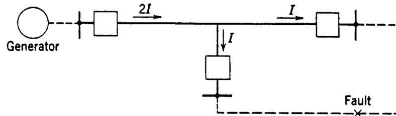
**Fig. 5. A situation in which directional relaying will not prevent reduced sensitivity.**
