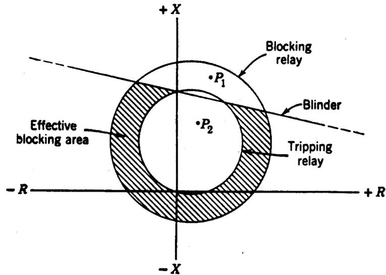
**Fig. 14. R-X diagram of the conditions of Fig. 13.**
