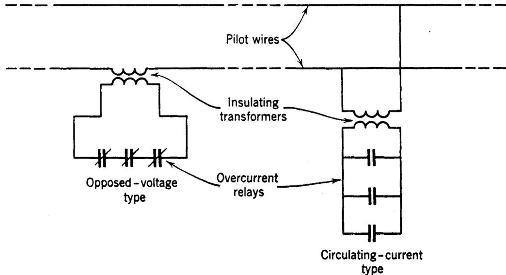
Fig. 2. Blocking-terminal technique.
