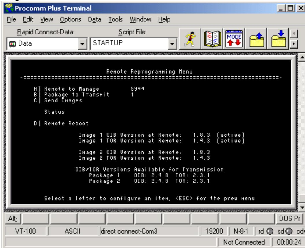
From this menu, you should choose the appropriate firmware package you wish to reprogram the remote with. In the case of an upgrade to 2.3.2 AP Firmware, choose the package labeled **OIB: 2.4.8** and **TOR 2.3.1**. These packages are the firmware that is associated with AP revision 2.3.1.
