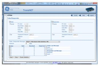
Used with two RF connected devices, the Poller and Responder capability is used to test data transfers via **Serial** or **IP** connection, depending on devices.
