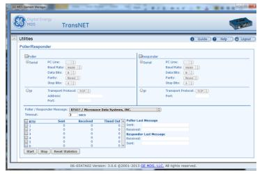
With two RF connected devices, the Poller and Responder capability is used to test data transfers via **Serial** or **IP** connection, depending on the devices used.
