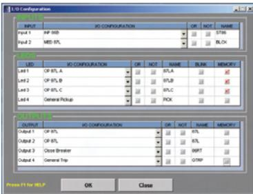
Input, output and LED configuration can be performed using EnerVista software
