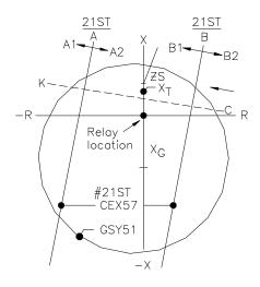
Fig. 2. Typical characteristic CEX57E with GY51A for out-of-step tripping
