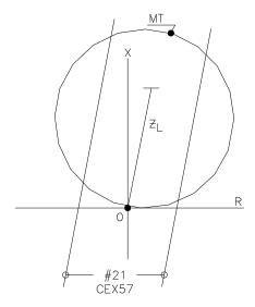
Fig. 1. Typical characteristic CEX57D or CEX57F as a blinder
