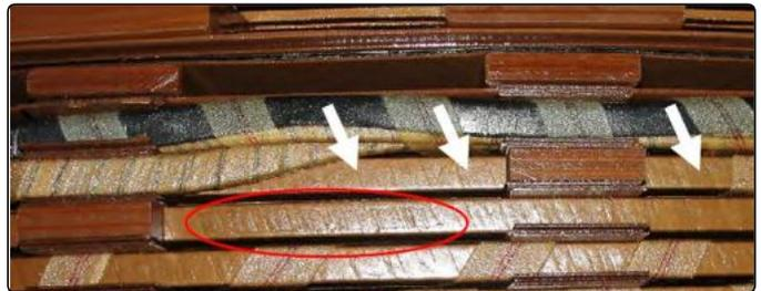
**Figure 3:** Paper sampling locations must be chosen according to the accessibility and rebuilt feasibility. Locations should be reasonably representative of winding temperature conditions or hot spot conditions.
