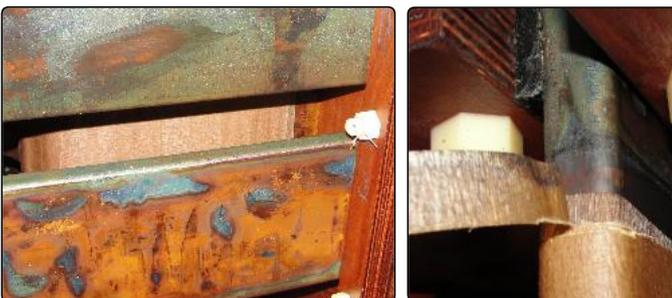
**Findings:** Copper sulphide formed on copper busbar and in the wraps of the paper insulation on copper conductors.
