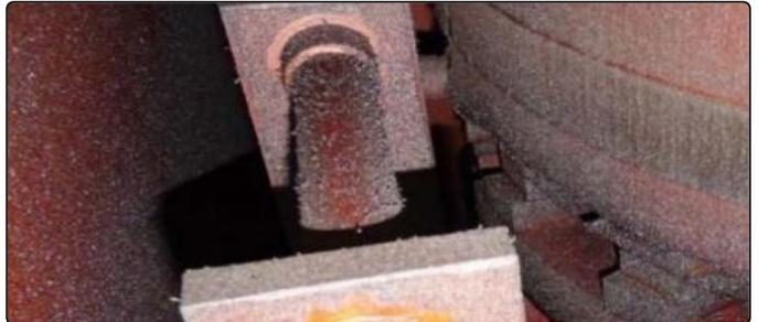
**Findings:** Sludge formation and aggregated particles aligned in a direction perpendicular to the surface, following the localized electrical field gradient.
