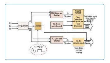
Figure 2 Phase comparison protection functional diagram
