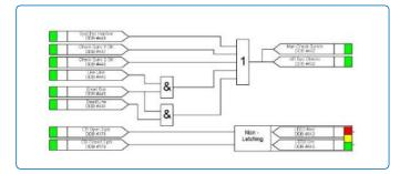
Figure 7 Programmable scheme logic
