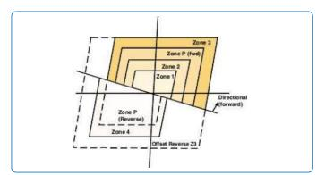
Figure 5 Quadrilateral characteristics
