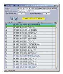
Record the operation of the internal T60 elements and external connected devices with 1ms timestamped accuracy to identify the Sequence of Operation of station devices during transformer faults and disturbances.
