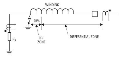
Faults close to the neutral point of a wye-connected winding does not generate adequate fault current for elements to detect. Restricted ground fault protection provides sensitive ground fault detection for low-magnitude fault currents.
