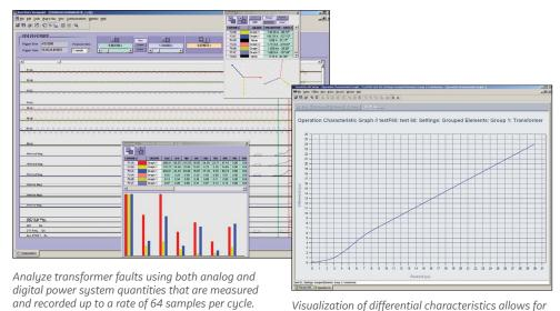
Visualization of differential characteristics allows for setting verification and operation troubleshooting.
