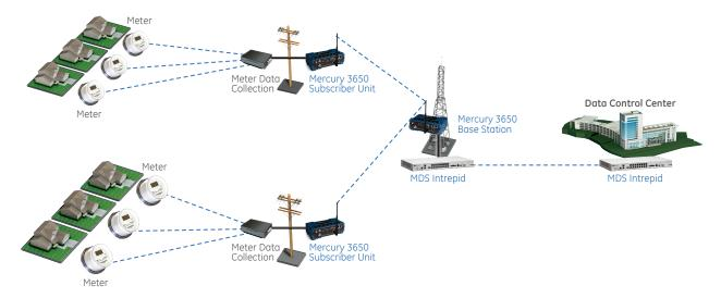
co-location and overlap of coverage without introducing self-inflicted interference. The MDS Mercury series has been specifically designed in three special packaging options for application flexibility and ease-of-use installation.
